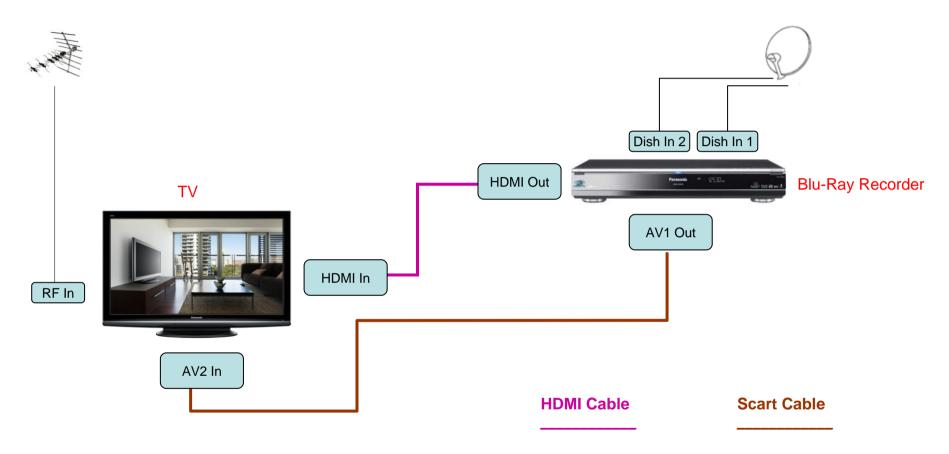
Connect a HDMI cable from the HDMI output on the Blu-Ray Recorder to the Television's HDMI input. \* For additional Q-Link features - Connect a Scart cable from the AV1 Out of the Blu-Ray Recorder to the AV2 input on the TV
