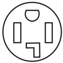
4-wire receptacle (14-30R)
