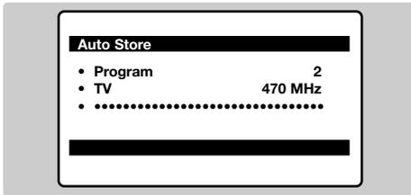
If the menu is not displayed, press and hold down the  $\triangleleft$ - and  $\triangleleft$ + keys on the TV set for 5 seconds to start the tuning.
