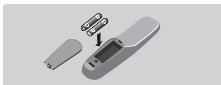
Insert the two R6-type batteries (supplied) making sure that they are the right way round. Check that the mode selector is set to TV. The batteries supplied with this appliance do not contain mercury or nickel cadmium. If you have access to a recycling facility, please do not discard your used batteries (if in doubt, consult your dealer). When the batteries are replaced, use the same type.
