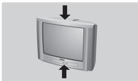
The VOLUME - + (-  $\triangleleft$  +) keys are used to adjust sound levels. The PROGRAM - + (- **P** + or - +) keys are used to select the required programmes. To access the menus, simultaneously hold down the  $\triangleleft$  - and  $\triangleleft$  + keys. The PROGRAM - + keys may then be used to select an adjustment and the -  $\triangleleft$  + keys to make that adjustment. To exit from the menus, hold down the 2  $\triangleleft$  - and  $\triangleleft$  + keys.
