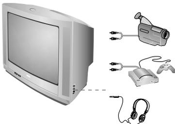
Depending on the versions, the connectors are located on the front (sometimes under a flap) or on the right-hand side of the TV set. Make the connections as shown opposite. With the **AV** key, select AV.
