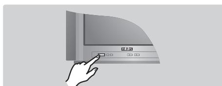
To switch on the set, press the on/off key. A red indicator comes on and the screen lights up. Go straight to the chapter Quick installation on page 4.
