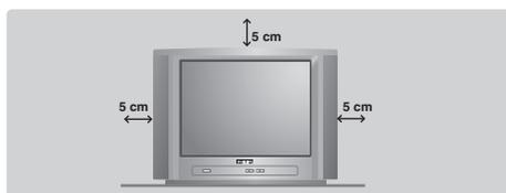
Place your TV on a solid, stable surface, leaving a space of at least 5 cm around the appliance. To avoid accidents, do not put anything on the set such as a cloth or cover, a container full of liquid (vase) or a heat source (lamp). The set must not be exposed to water.
