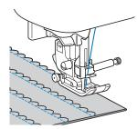
Unfold the fabric, and then iron the tucks down to one side.
