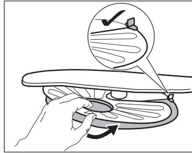
7. Reassemble the filters (B) and (C).
