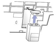
Insert and place the battery in the battery compartment.
