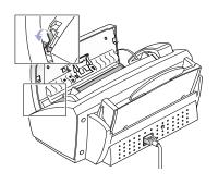
**Disassemble the White Roller.** At the right-hand end of the White Roller there is a bushing that is secured with a small white tab. Push the tab slightly inward, then rotate towards you. Then pull up the right-hand part to take it out.
