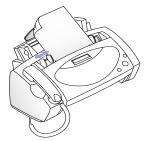
Feed the document into the machine. The automatic document feeder pulls in the page. If necessary, press RCV.Mode/Contrast to choose the desired contrast for the document.
