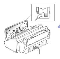
**Clean the ADF Rubber piece** at the back of the Control Panel, too.
