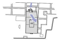
Connect the new battery to the clips.
