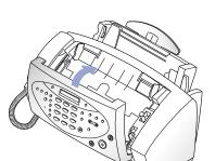
**Replace the roller in reverse order**, and then close the Control Panel firmly until it clicks into place.
