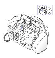
Open the Control Panel and Cartridge Compartment Cover and remove the Cartridge.
