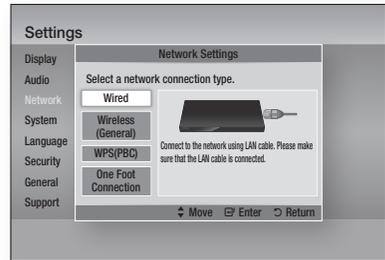
2. Press the **ENTER** button. The Network Status screen appears. The player connects to the network after the network connection is verified.
