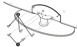
1. Connect the Guide Stand to the Stand using four screws (M4 X L12) as shown.
