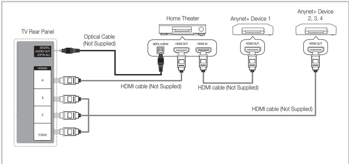
1. Connect the **HDMI IN (1(DVI), 2, 3 or 4)** jack on the TV and the **HDMI OUT** jack of the corresponding Anynet+ device using an HDMI cable.
