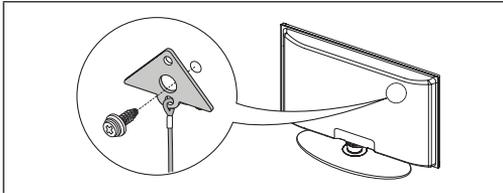
2. Firmly fasten the screw to the wall or cabinet where the TV is to be installed. Tie the TV-Holder attached to the TV and the screw fastened on the wall or cabinet so that the TV is fixed.
