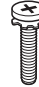
Viti del supporto 4EA, M4 x L14 (Solo 39/42/47/50LB57**, 39/42/47/50/55LB58**- ZA/ZB/ZG/ZJ, 42/47/50/55/60LB58**-ZM, LB61**)
