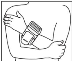
2. Help the patient to take the measuring position as shown. The arms should remain close to the body. Make sure the appliance is positioned approximately at the person's heart level. Move the forearm of the patient up or down (see illustration) in the direction of the arrow.
