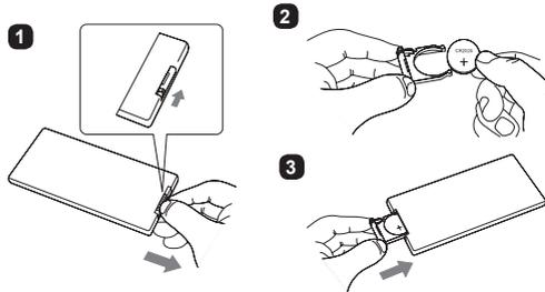
Replacing the battery (CR2025)
