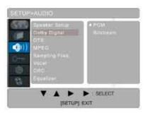
In this menu you can set the format for the audio output that matches the output device (TV, amplifier, etc.)
