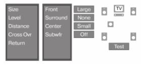
In the Speaker Setup sub-menu you can set the size, volume, delay and frequency range for each individual channel.
