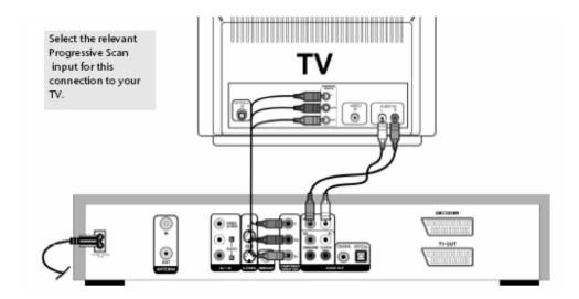
To playback the Progressive Scan image you have to press the NTSC/PAL button on the remote control to select the Progressive Scan format. You can only select this format if the YCrCb On
