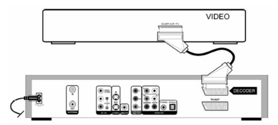
You can also connect a decoder or set-top box (e. g. a Canal+ decoder) to the SCART input. To do so set the DECODER entry in the SETUP>CHANNEL SETUP menu to ON ("Decoder", Page 22).
