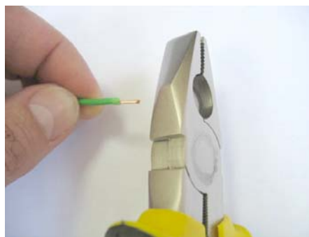
Figure 1.15 - Dénudez 6mm (0.25 pouces) d'isolation from the wire end
