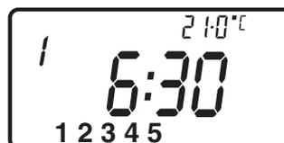
Returning to RUN Mode – press **PROG** until colon flashes in display.
