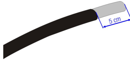
Figure 6: De-sheathing the CAT cable
