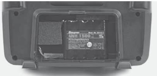
Remove the battery, then carefully pull on the power lead to disconnect the transmitter battery connector.
