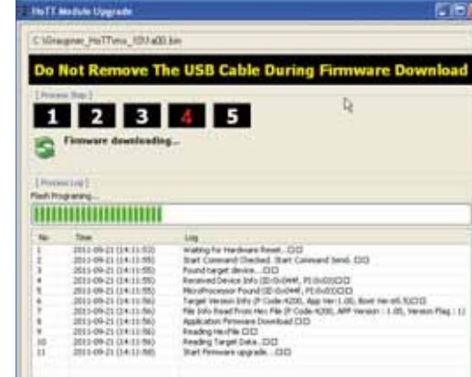
Do not interrupt the update process until the progress bar has reached the right-hand margin, and you see the message “Firmware Download Success” - also a brief buzzer sound appears and the STATUS-LED of the transmitter changes from orange to green:
