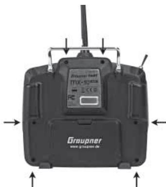
Hold the two case sections together with your hand, and turn the unit over to allow these six screws to fall out onto the table. Now carefully raise the case back and fold it open to the right, as if you were opening a book.
