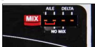
„Delta/FW“: The aileron and elevator rudder is controlled by one servo per wing half, connected on channel 2 and 3. The coupling function for the aileron and elevator control is performed automatically by the transmitter mixer.
