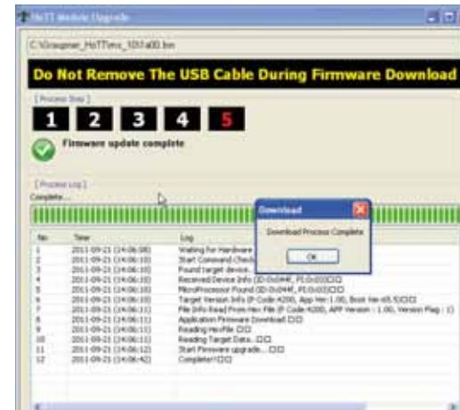
Click on "OK", then switch the transmitter off and finally disconnect the PC or laptop.
