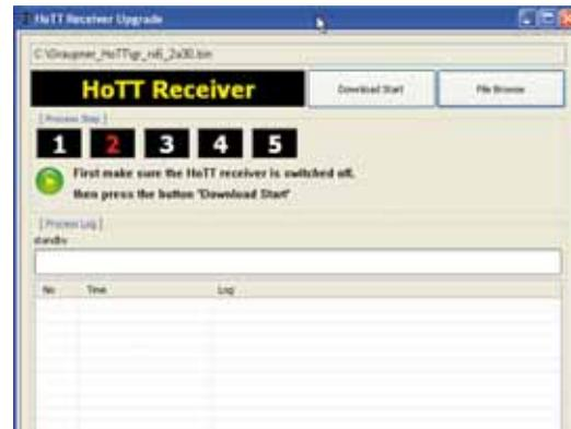
The firmware files are present in a product-specific encoded form, i.e. if you inadvertently select a file which does not match the product (e.g. transmitter update file instead of receiver update file) the pop-up window "Product code error" appears, and the update process cannot be started.
