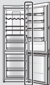
Potential pinch point
