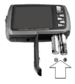
Insert 2 x AAA (1.5V) batteries. Alkaline batteries recommended (not included).
