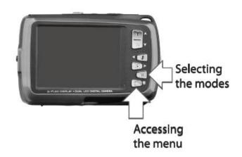
When powering the camera ON for the first time the camera will take you through the INITIAL CAMERA SETUP.
