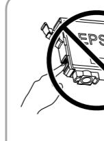
Do not touch the sections shown in the illustration of the cartridge.
