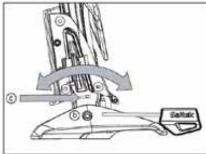
Insert the adjustment tool in the locking nut (d) and turn counter-clockwise to unlock the head mechanism. Move to the required angle and lock by turning the locking nut clockwise.
