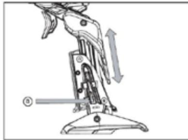
Insert the adjustment tool in the locking nut (b) and turn counter-clockwise. Press the locking pin (c) in and move the stick forward or backwards to the required angle. Lock by turning locking nut (b) clockwise.
