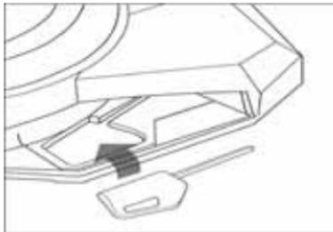
Press the locking switch (a) and move the stick up or down to adjust the height.
