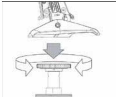
Remove the adjustment tool from the compartment on the stick base.
