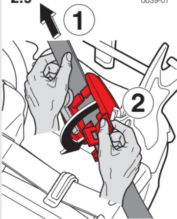
Tighten the upper belt (1) slightly and close the **red** belt clip (2). Then tighten the belt once again.
