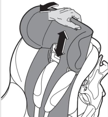
Grasp the head support at the top and pull it forwards. You can then set it to the height that is right for your child. There are six possible different positions.
