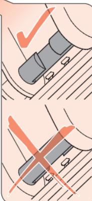
Position the upper belt (diagonal belt) in the opening of the ratchet shaft and into the guide mechanism behind it.
