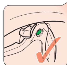
Always check that when the seat shell is inserted a **green dot** is visible **on both sides** through the opening on the sidepieces. This indicates that the seat is installed correctly.
