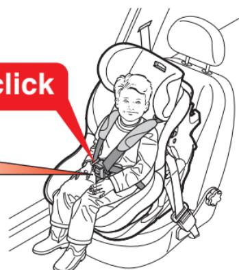
Fit both belt parts together (see illustration) and push them into the belt buckle so that they engage with an audible "click".
