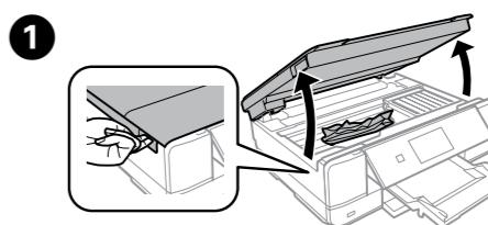
Open the scanner unit and remove all of the paper inside, including any torn pieces.
