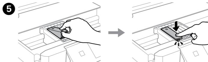
Insert the ink cartridge diagonally into the cartridge holder and gently push it down until it clicks into place.
