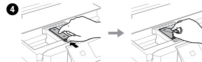
Push the tab to unlock the ink cartridge holder and then remove the cartridge diagonally.
