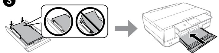
Align the edges of the paper. Keep the cassette flat and insert it back into the printer carefully and slowly.
