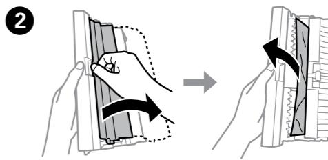
Open the rear cover and carefully remove the jammed paper.
