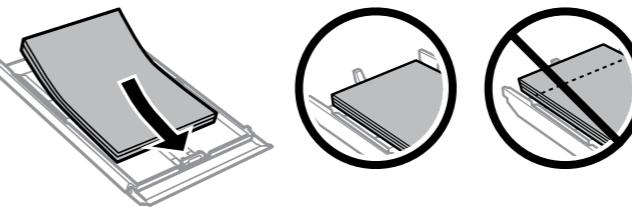
Load paper toward the edge guide with printable side face-down, and check that the paper is not sticking out from the end of the cassette.
