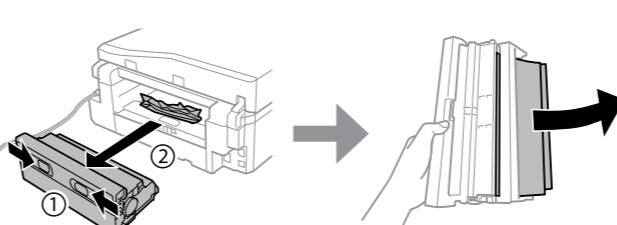
Pull out the rear cover and carefully remove the jammed paper.
