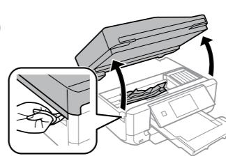
Open the scanner unit and remove all of the paper inside, including any torn pieces.
