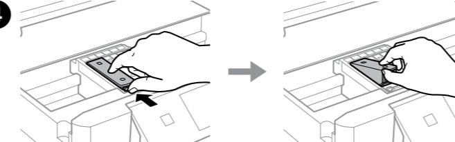
Push the tab to unlock the ink cartridge holder and then remove the cartridge diagonally.
