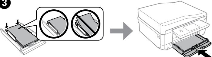
Align the edges of the paper. Keep the cassette flat and insert it back into the printer carefully and slowly.
