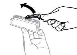
Remove the cap from the new cartridge.
