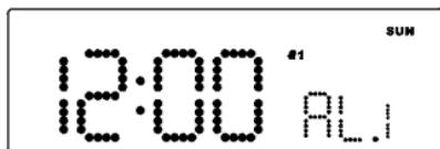
Display Show Alarm 1 wake up by Buzzer
