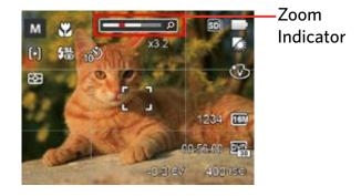
When the optical zoom reaches the threshold as digital zoom, release and turn the zoom lever to T to switch between the optical zoom and digital zoom.
