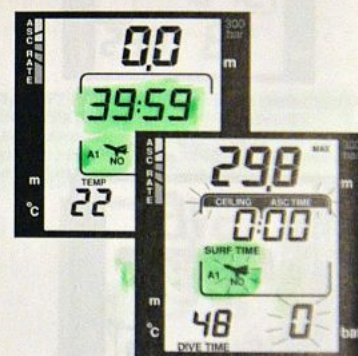
Fig. 3.20 AFFICHAGES SURFACE APRES DECOMPRESSION INCOMPLETE
