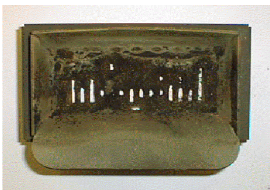
Photo 7: pot de combustion encrassé
