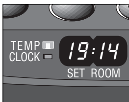
F: The required temperature on the left, the measured temperature on the right.
