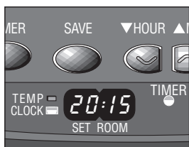
G: The TIMER indicator light indicates that the timer function has been switched on.
