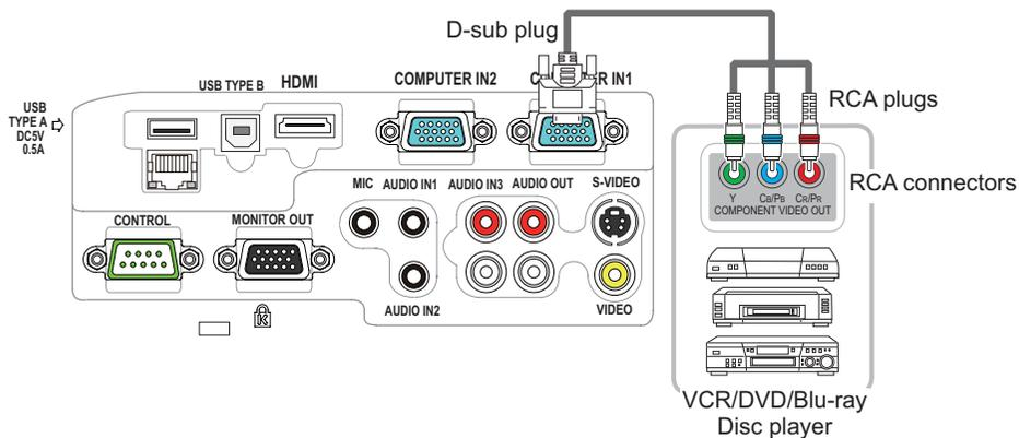
To input component video signal to the **COMPUTER IN1** or **IN2** port of the projector, use a RCA to D-sub cable or adapter.
