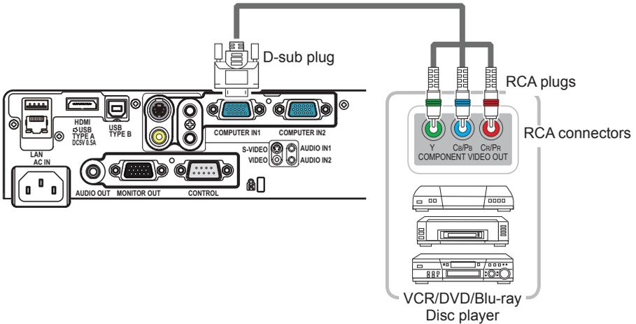
To input component video signal to the **COMPUTER IN1** or **COMPUTER IN2** port of the projector, use a RCA to D-sub cable or adapter.
