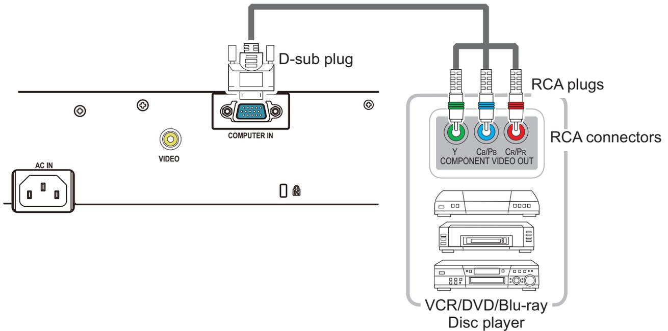
To input component video signal to the **COMPUTER IN** port of the projector, use a RCA to D-sub cable or adapter.
