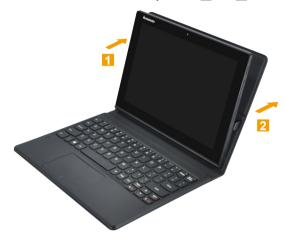
2 Remove the tablet in the direction shown by arrow **3**.
