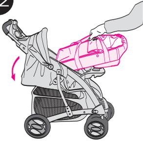
Fully recline seat back and place carrycot into pushchair as shown. Reverse the canopy and wrap the tray cover around the bottom of tray as shown in 33.
