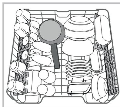
Several dishwasher models are fitted with tip-up sectors\*. They can be used in a vertical position when arranging tea/dessert saucers or in a lower position to load bowls and food containers.
