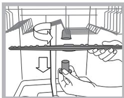
To remove the upper spray arm, turn the plastic locking ring in an anti-clockwise direction. The upper sprayer arm should be replaced so that the side with the greater number of holes is facing upwards.
