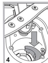
After cleaning the filters, re-place the filter assembly and fix it in position correctly; this is essential for maintaining the efficient operation of the dishwasher.
