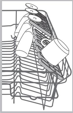
Wine glasses can be placed safely in the tip-up compartments by inserting the stem of each glass into the corresponding slots. For optimum drying results incline the tip-up compartments more. To change the inclination, pull up the tip-up compartment, slide it slightly and position it as you wish.
