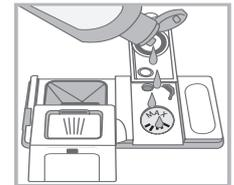
1. Open the dispenser "D" by pressing and pulling up the tab on the lid;
