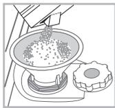
1. Remove the lower rack and unscrew the container cap (anticlockwise).
