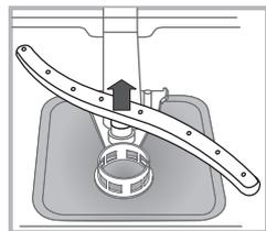
The lower spray arm can be removed by pressing on the side tabs and pulling it upwards.
