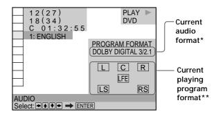
\* "PCM," "DTS," "DOLBY DIGITAL" or "MPEG" is displayed. In case of "DOLBY DIGITAL," the channels in the playing track are displayed by numbers as follows:
