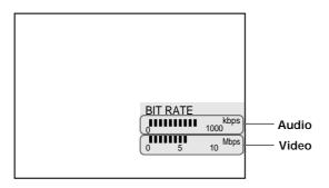
Bit rate refers to the amount of video/audio data per second in a disc. The higher the bit rate, the larger the amount of data. When the bit rate level is high, there is a large amount of data. However, this does not always mean that you can get higher quality pictures or sounds.
