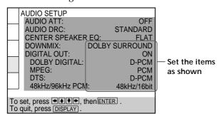
When you have made the connections using an optical or coaxial digital connecting cord, do not set "DOLBY DIGITAL" to "DOLBY DIGITAL," "MPEG" to "MPEG," "DTS" to "DTS" and "48kHz/96kHz PCM" to "96kHz/24bit." If you do, a loud noise will suddenly come out from the speakers, affecting your ears or causing the speakers to be damaged.
