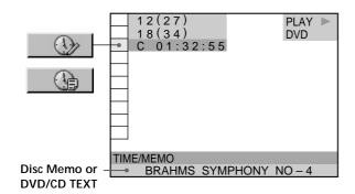
You can select "TIME/MEMO" or "TIME/TEXT" directly Press TIME/TEXT on the remote. To display DVD/CD TEXT or Disc Memo, press TIME/TEXT until DVD/CD TEXT or Disc Memo is displayed.
