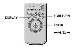
1 Press DISPLAY and select "SETUP" using ↑/↓.
