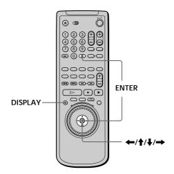
1 When the player is in stop mode, press DISPLAY and select "SETUP" using ↑/↓.
