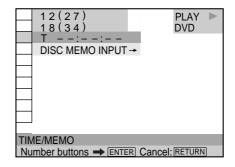
2 Select "DISC MEMO INPUT→" and press ENTER. The DISC MEMO INPUT display appears.
