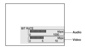
Bit rate refers to the amount of video/audio data per second in a disc. The higher the bit rate is, the larger the amount of data. When the bit rate level is high, there is a large amount of data. However, this does not always mean that you can get higher quality pictures or sounds.
