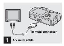
→ Connect the A/V multi cable (supplied) to the multi connector of the camera and the audio/video input jacks of the TV.
