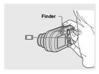
The finder is convenient when you want to save battery power, or when it is difficult to confirm the image using the LCD screen. Each time you press [\_], the display changes in the following order.
