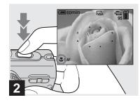
Center the subject in the frame. Press and hold the shutter button halfway down to focus on, then press the shutter button fully down.
