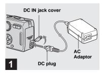
Open the DC IN jack cover and connect the AC Adaptor (supplied) to the DC IN jack of your camera.
