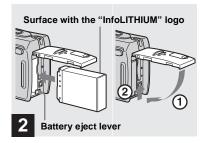
→ Install the battery pack, then close the battery/"Memory Stick" cover.
