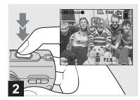
Center the subject in the frame. Press and hold the shutter button halfway down to focus on, then press the shutter button fully down.
