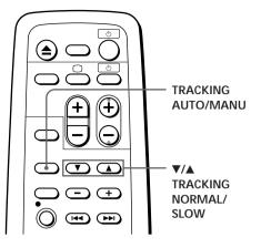
distortion should disappear as you press one of the two buttons. If you cannot get a clear picture with manual adjustment, press TRACKING AUTO/MANU to return to automatic adjustment.
