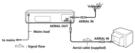
Disconnect the aerial cable from your TV and connect it to AERIAL IN on the rear panel of the VCR.
