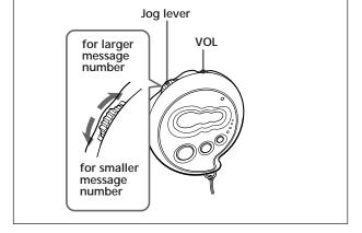
1 Move the jog lever to display the desired message number. (To change the number rapidly, keep holding the lever.)
