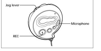
1 Press REC and speak into the built-in microphone. "REC" appears while recording.
