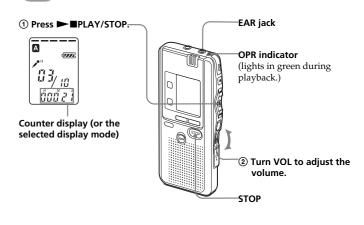
After playing back one message, the unit stops at the beginning of the next message. When the continuous play function is set to "ON" (see the reverse side), the unit stops after playing all messages in a folder. When the last message on a folder has been played back, the unit stops at the beginning of the last message
