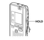
Slide the HOLD switch in the direction of the arrow. "HOLD" will flash three times indicating that all the functions of the buttons are locked.
