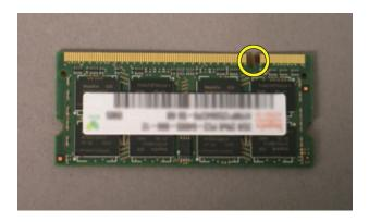
2 Holding the card by its edges, slide it all the way into the slot, and then gently push downward on it to snap it into place.
