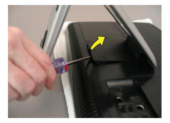
7 Use a Phillips screwdriver to remove the three screws holding the stand.
