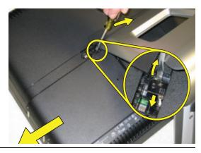
**9** Loosen the screw at the front of the hard disk drive cage.
