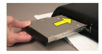
2 Slide the CD/DVD drive assembly all the way into the computer until the bezel is flush with the side of the computer and the drive locks into place.
