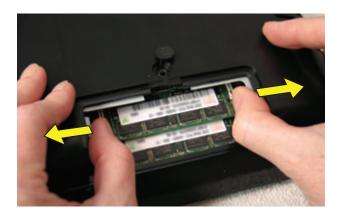
11 Holding the card by its edges, remove it from the compartment.
