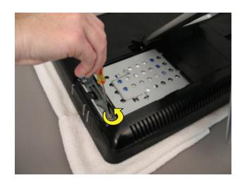
10 Lift up the metal handle on the hard disk drive cage and pull it firmly toward you to remove the hard disk drive cage from its bay.
