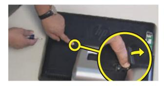
7 Use a Phillips screwdriver to remove the hard disk drive cover screw.
