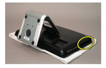
**7** Use your finger to lift up the rubber cover over the screw.
