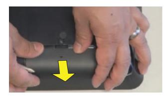
10 Use your fingers to press outwards on the tabs on the left and right sides of the top memory card to release it.
