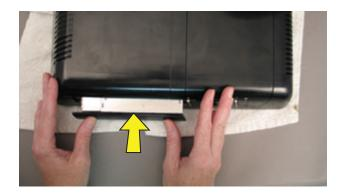
Using a Phillips screwdriver, replace and tighten the CD/DVD drive screw.
