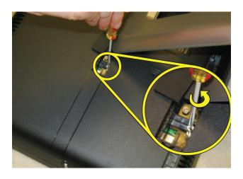
8 Insert a small flathead screwdriver gently into the notch and use a levering motion to disengage the CD/DVD drive assembly.
