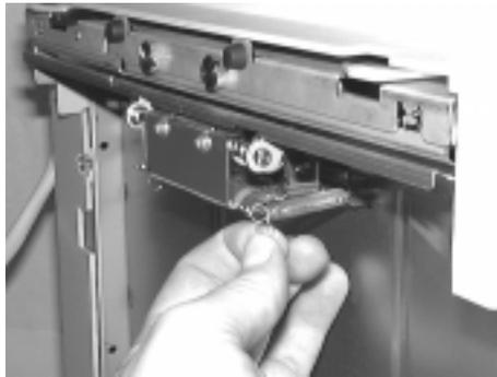
*Figure 4-70 Installation des ressorts*
