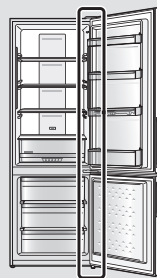
Potential pinch point
