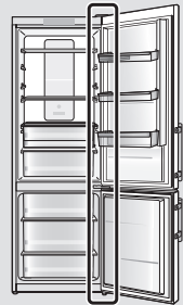
Potential pinch point
