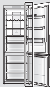
Potential pinch point
