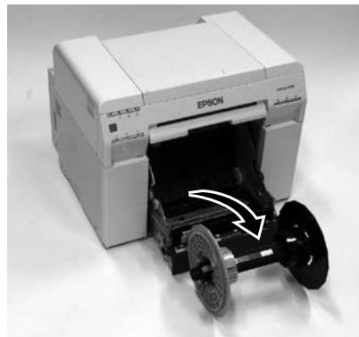
**Remove the spindle unit.**
