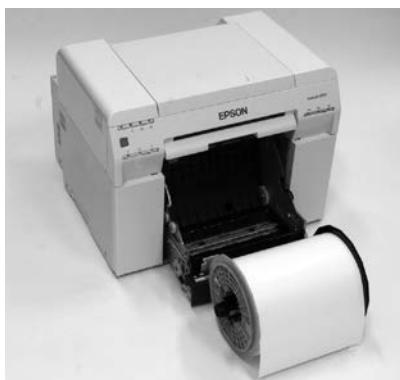
**Hold the spindle unit in the direction shown above, and then place it in front of the roll paper feeder.**
