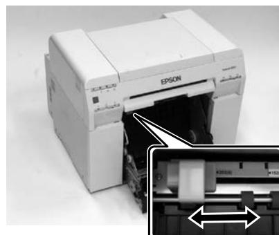
**Match the inner edge guide on the roll paper feeder to the size of the paper.**
