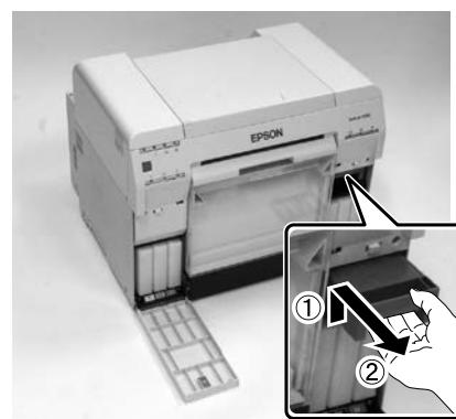
**Remove the Maintenance cartridge carefully without tilting. Push it up, and then pull it out.**
