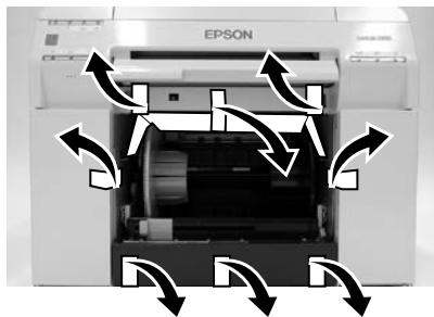
**Remove the protective cardboard and tape from inside of the roll paper feeder.**
