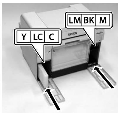
**Remove the ink cartridges from the bag, and insert them fully into the printer.**
