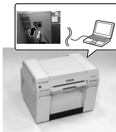
**Turn off the printer, and then connect the USB cable to the printer and the computer.**
