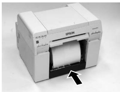
**Push the roll paper feeder into the printer.**
