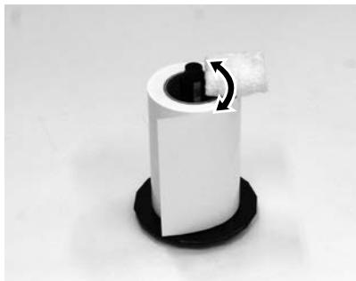
**Wipe the edge of the paper with a soft cloth several times to remove any dirt such as paper powder.**
