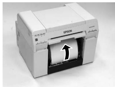
**Carefully roll the paper into the printer to take up any slack.**
