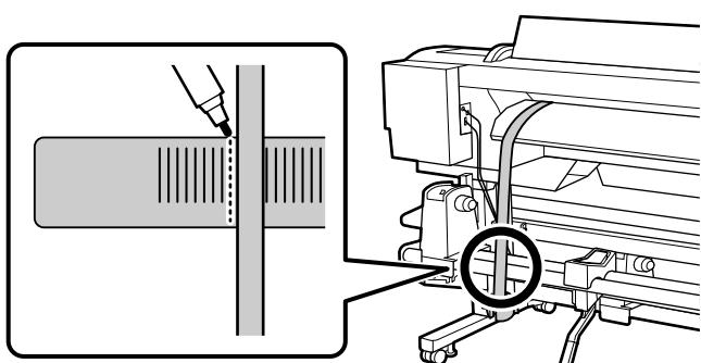
Pull the film straight down, and place it over the label on the front bar of the Media Feeding Unit. Use a marker such as an oil-based pen to mark the left end position of the film on the label.
