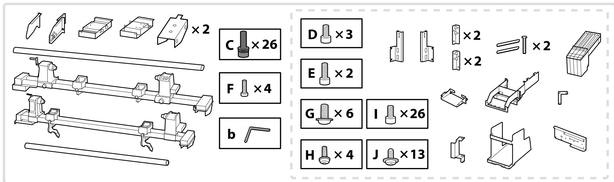
The dashed border indicates parts for the Ink Supply System and the Ink Supply System Cover.
