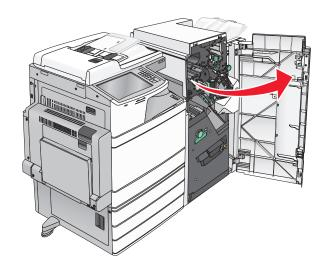
2 Press the handles of the staple cartridge to the right, and then take the staple cartridge unit out of the finisher.
