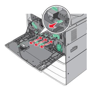
Slide the printhead wipers back into place.
