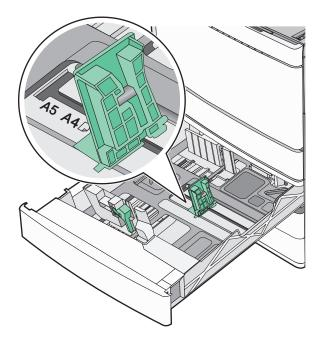
**2** Squeeze and then slide the width guide to the correct position for the paper size loaded.
