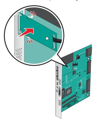
Connect the ISP solution interface cable into the receptacle of the system board.
