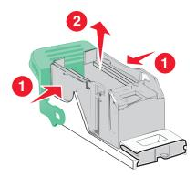
7 Insert the front side of the new staple case into the staple cartridge, and then push the rear side into the cartridge.
