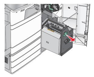
Lift the inside cover. If the paper is jammed in the rollers, then rotate knob G8 counterclockwise, and then remove the jammed paper.
