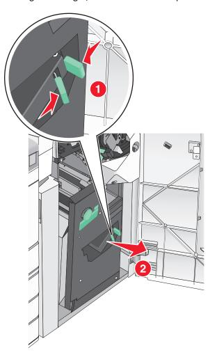
${\bf 3} \ \ \mbox{Hold the tabs on both sides of the staple cartridge}.$
