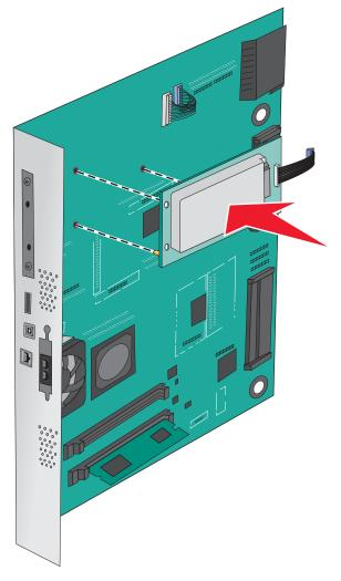
**b** Use the two provided screws to attach the printer hard disk mounting bracket.
