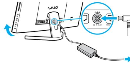
Adjust the angle of the screen to locate the DC IN port behind the foot stand. Route the AC adapter cable through the hole in the foot stand and plug it into the DC IN port. Plug the power cord into the AC adapter, then plug it into an AC outlet.
